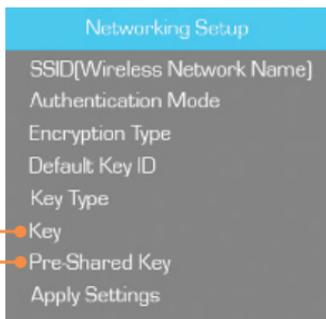
9. Select **Apply Settings** using the down arrow on the remote control. Then press **Enter**.
