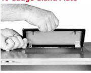
Constructed of 16 gauge steel. Gland plates will maintain UL/CSA Type 12 integrity while providing a removable cable egress and entry plate. Easily installed by cutting a rectangular opening in the enclosure. Finish is ANSI 61 gray polyester powder paint.
