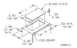
Constructed of 12 gauge steel and designed for use with 10 gauge and 12 gauge enclosures. Provides a removable cable egress and entry plate while maintaining UL/NEMA integrity of the enclosure. Gasket with pressure-sensitive adhesive is included to be applied after desired modifications are completed. Finish is ANSI 61 gray polyester powder paint. Maintains UL/NEMA Type 4 and Type 12 if properly installed in a Hoffman enclosure.
