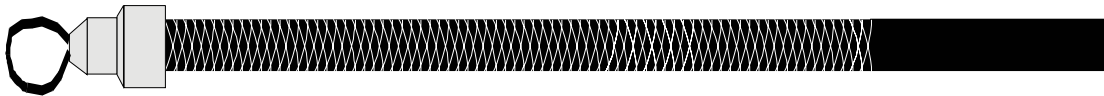
Figure 3: Completed setup on outside plant ribbon central loose tube or outside plant bundled central loose tube cable with grip applied over cable
