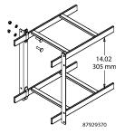
Allows stacking any width of ladder rack runways 12 in. (305 mm) above each other. Each kit contains two complete stacking brackets with all necessary hardware. Use one kit at least every 5 ft. (1.5 m). Brackets and fasteners made of plated steel.
