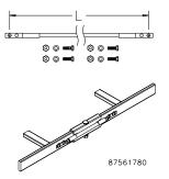
Fastens across splices to provide a secure ground between sections of ladder rack. Made of #6 AWG x 7 strand wire with green THW insulation and two-hole compression lugs mounted on each end. Includes fasteners.
