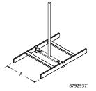
Threaded rod and bracket supports center of ladder rack from ceiling. Kit includes heavy-duty ladder rack cross member, 5/8-in. threaded rod, two J-bolts, protected sleeve and 5/8-in. nut. Use one kit at least every 5 ft. (1.5 m). Made of plated steel.
