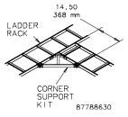
Provides additional support for 90-degree ladder rack junction. Made of steel with a painted or plated finish.
